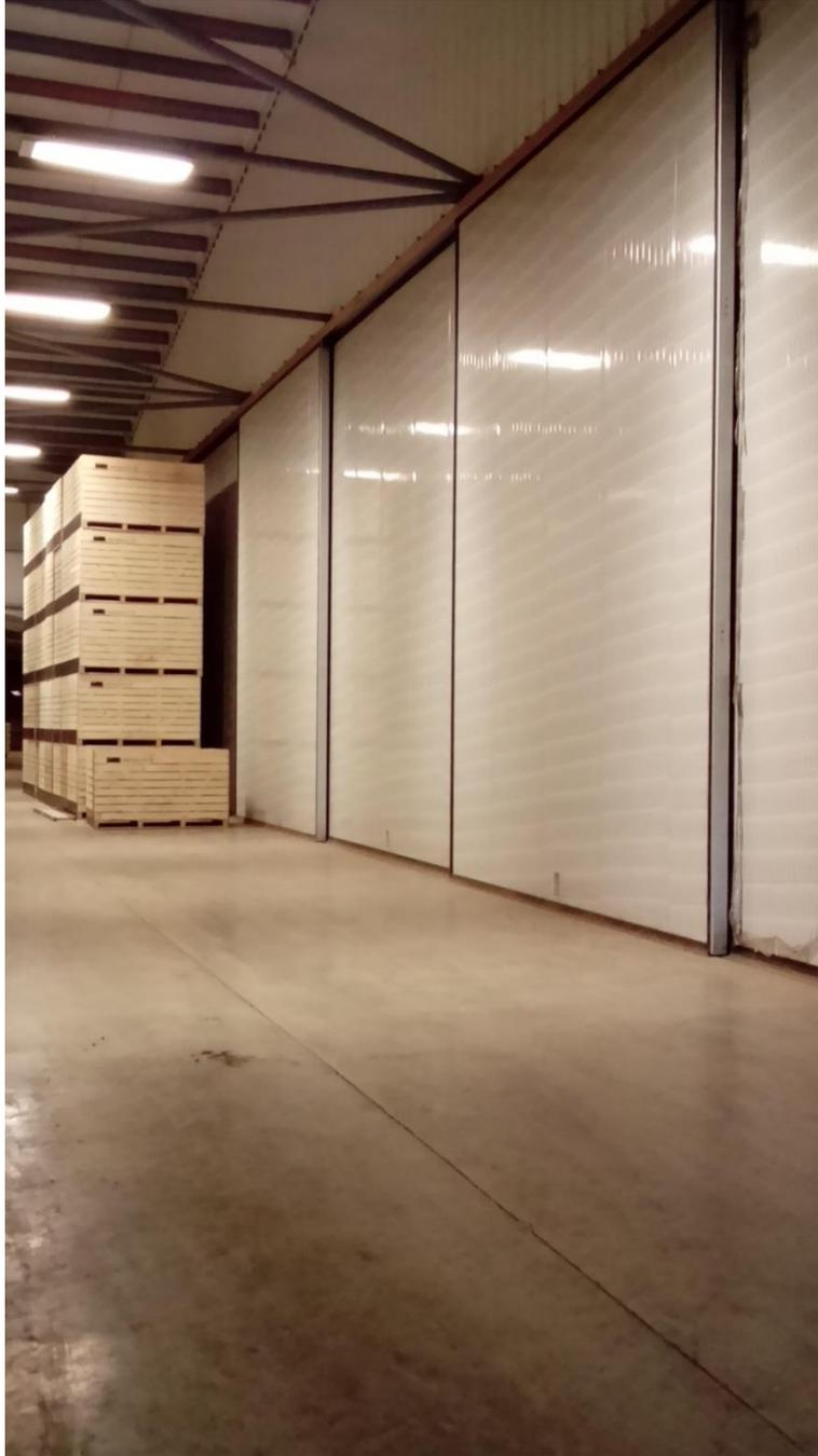
Figure 2: Doors across stack ends to avoid 'backfill'
