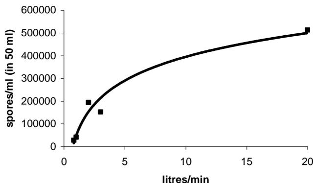
FIGURE 2 THE RELATIONSHIP BETWEEN THE NUMBER OF SPORES RECOVERED FROM THE IMPINGER AT VARYING FLOW RATES.
