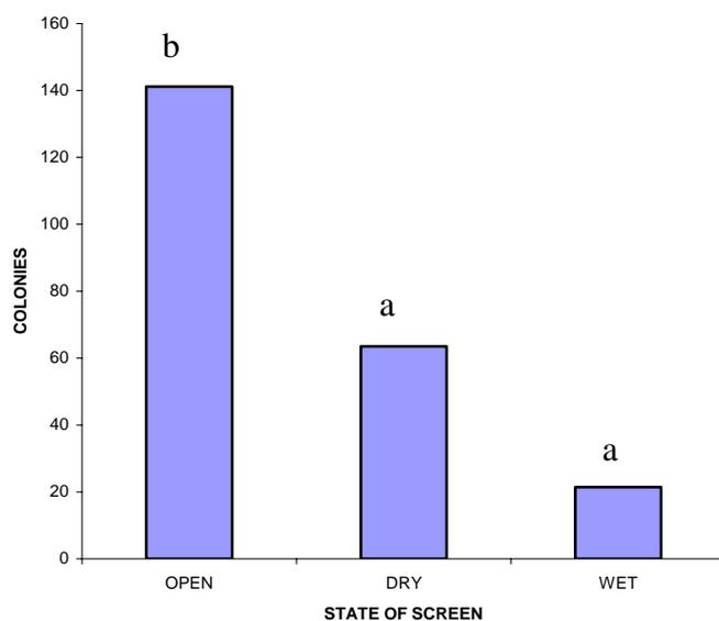
FIGURE 3 THE NUMBER OF COLONY FORMING UNITS RECOVERED ON PETRI DISHES POSITIONED BEHIND THE HUMIDIFIER UNIT WITH HUMIDIFIER SCREEN REMOVED (OPEN); SCREEN INSTALLED DRY; AND SCREEN INSTALLED WET (I.E. NORMAL OPERATION).  $LSD_{(P=0.05)} = 49$  (14 df). Different letters above the columns indicate a significant difference at  $P < 0.05$ .
