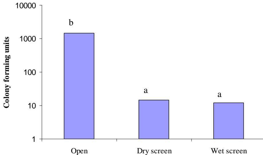
FIGURE 4 THE LOG NUMBER OF COLONY FORMING UNITS OF *FUSARIUM SULPHUREUM* RECOVERED ON PETRI DISHES POSITIONED BEHIND THE HUMIDIFIER UNIT WITH HUMIDIFIER SCREEN REMOVED (OPEN); SCREEN INSTALLED DRY; AND SCREEN INSTALLED WET (I.E. NORMAL OPERATION).  $LSD_{(P=0.05)} = 911$  (14 df). Different letters above the columns indicate a significant difference at  $P < 0.05$ .
