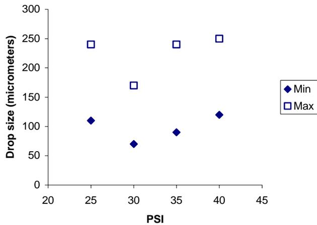
FIGURE 1 THE RELATIONSHIP BETWEEN THE SIZE OF WATER DROPLET PRODUCED BY AIRBRUSH AND AIR PRESSURE.
