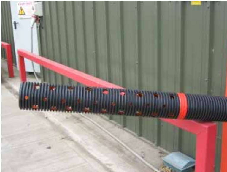
FIGURE 6. PERFORATION OF BASE OF SAMPLE PIPE TO ENCOURAGE UNIMPEDED MOVEMENT OF AIR AND CIPC THROUGH SAMPLES FOR ESTIMATION OF RE-DISTRIBUTION OF THE SPROUT SUPPRESSANT.
