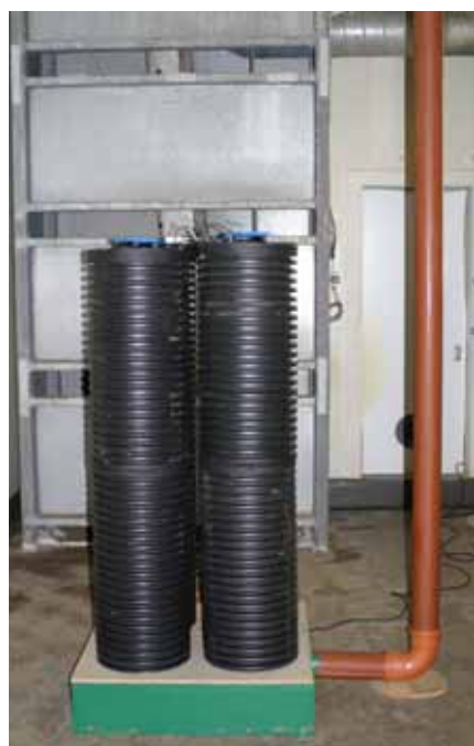
FIGURES 4 & 5. ARRANGEMENT OF PIPES WITH FANS IN CIPC REDISTRIBUTION TRIAL.
