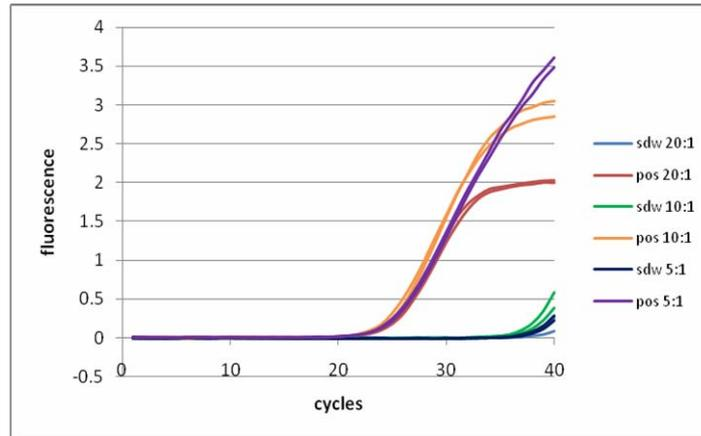
FIGURE 1. AMPLIFICATION PLOTS FOR LATE-PCR AMPLIFICATION OF PECTOLYTIC BACTERIA USING DIFFERENT PRIMER RATIOS. THE INTERCALATING DYE DETECTS DOUBLE-STRANDED AMPLIFICATION PRODUCTS, THE GENERATION OF WHICH REACHES A PLATEAU AT A LOWER LEVEL IF A MORE SYMMETRICAL PRIMER RATIO IS USED.
