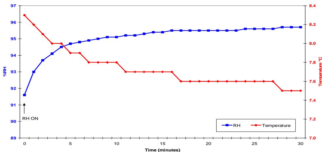
Figure 3. Case study 2: Bulk store ventilation with ultrasonic humidification illustrating cooling effect
