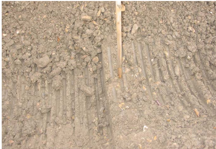
FIGURE 17. SMEARED PAN CREATED BY PICK TINE BED-TILLER WORKING IN SOIL ABOVE IT PLASTIC LIMIT
